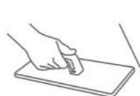
COMPRESSING THE TILE
